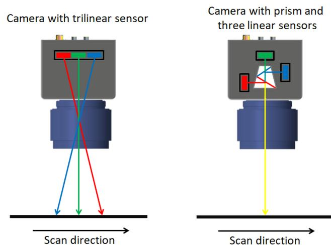
**Figure 1: Trilinear (left) versus prism-based (right) line-scan technology.**
