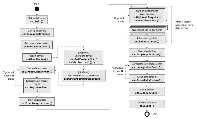
Depending on the type of the device it is possible to retrieve multiple data streams in parallel from the same device. This capability can be checked by using the "csiGetNumberOfDataStreams"-function which is described in the chapter 4.5 Functions related to image acquisition.
