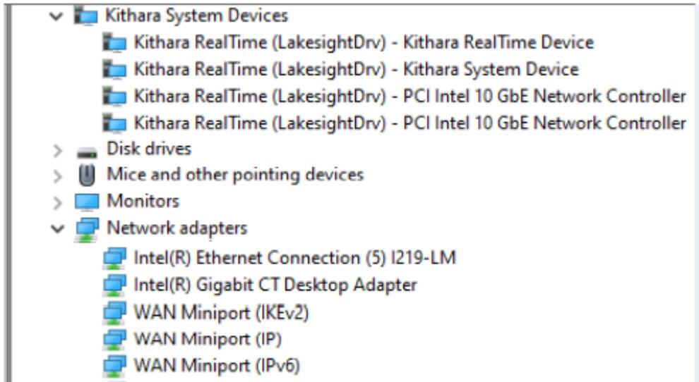
The network adapters used by Kithara can be found under Kithara now in the case above the two Intel 10 GbE network controllers.
