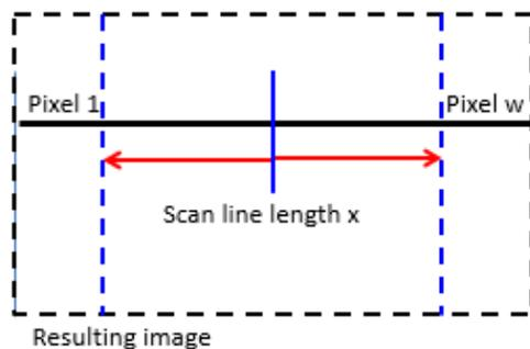
The camera captures an image from a ROI which is centered in the sensor.
