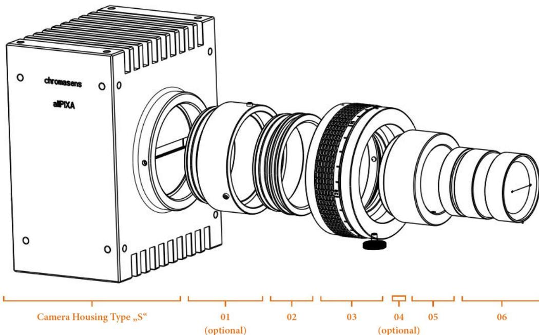
**Figure 20: configuration scheme (housing type S)**
