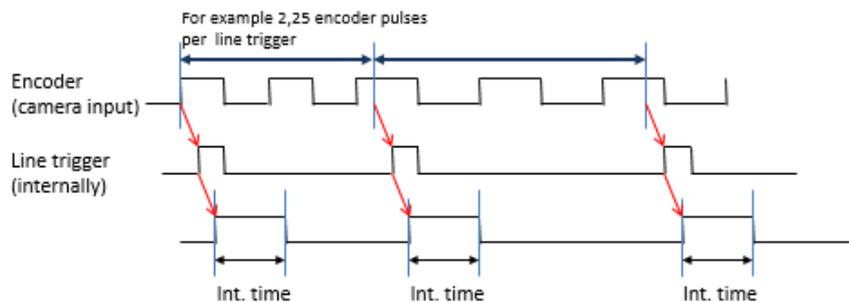
**NOTE** Minimum pulse duration of the line trigger or encoder has to be 5 pulses of the internal pixel clock of 85 MHz. Minimum pulse duration is 60ns. Otherwise, the pulse might be ignored due to debouncing within the camera.
