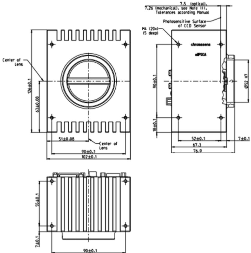
**Figure 2: Mechanical dimensions of the allPIXA camera**
