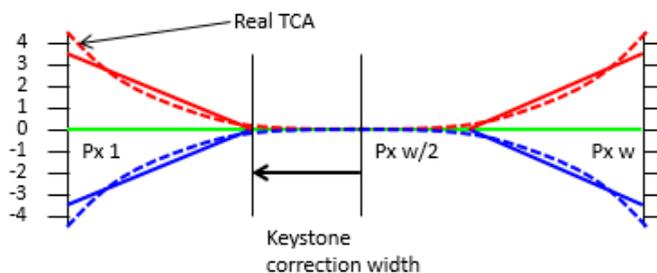
TCA (= Transversal Chromatic Aberration) is an objective-caused displacement of 3 colors increasing at the edge.
