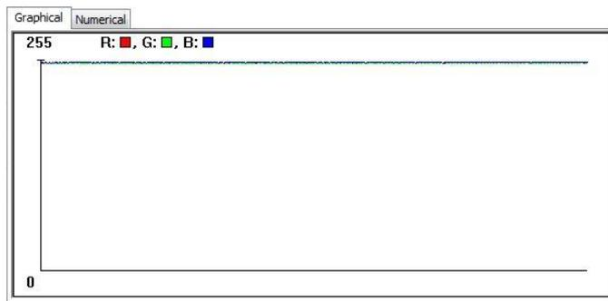
**Note:** At a later point, the image can be "desaturated" to a target value off, for example, 230 for a white paper by using a contrast adjustment of  $230/255=0,90$ .
