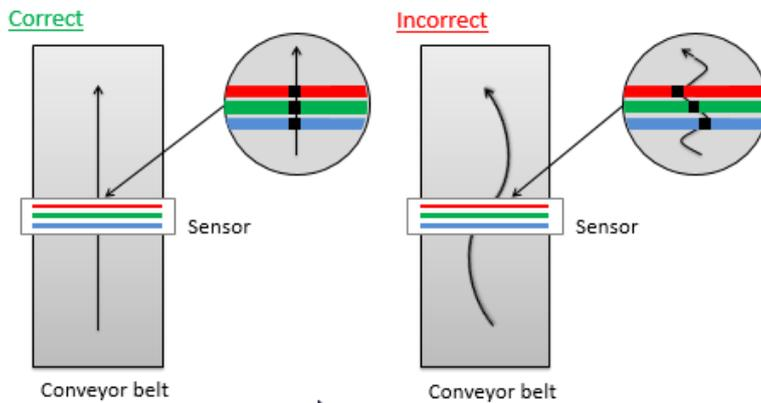
**Figure 27: Optimum conveying belt tracking**
