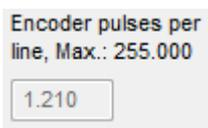
**NOTE** **Vertical image resolution** and **Integration time** have to be suitable to the speed of the transport. The time for one line (Speed divided by resolution) should be longer than the shortest possible integration time. In case of higher speed, the camera switches to free-running line mode.
