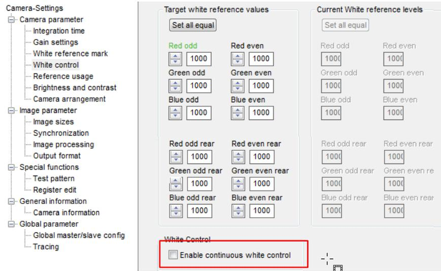
The screenshot shows the 'Camera-Settings' tree view on the left with 'White control' selected. The main panel displays 'Target white reference values' and 'Current White reference levels' for Red, Green, and Blue channels, both odd and even, and rear views. At the bottom, the 'White Control' section has the 'Enable continuous white control' checkbox checked, which is highlighted with a red box.
