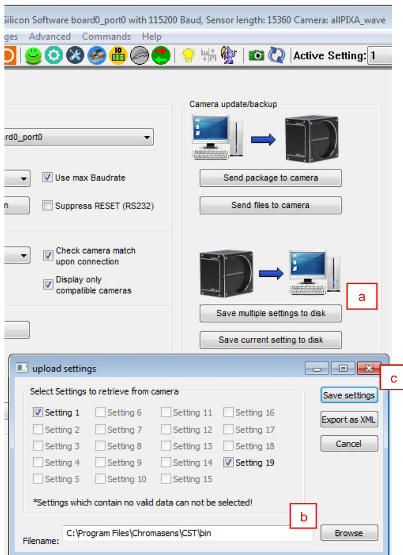
Settings are saved as single files in the specified folder. The setting number is appended to the specified filename.
