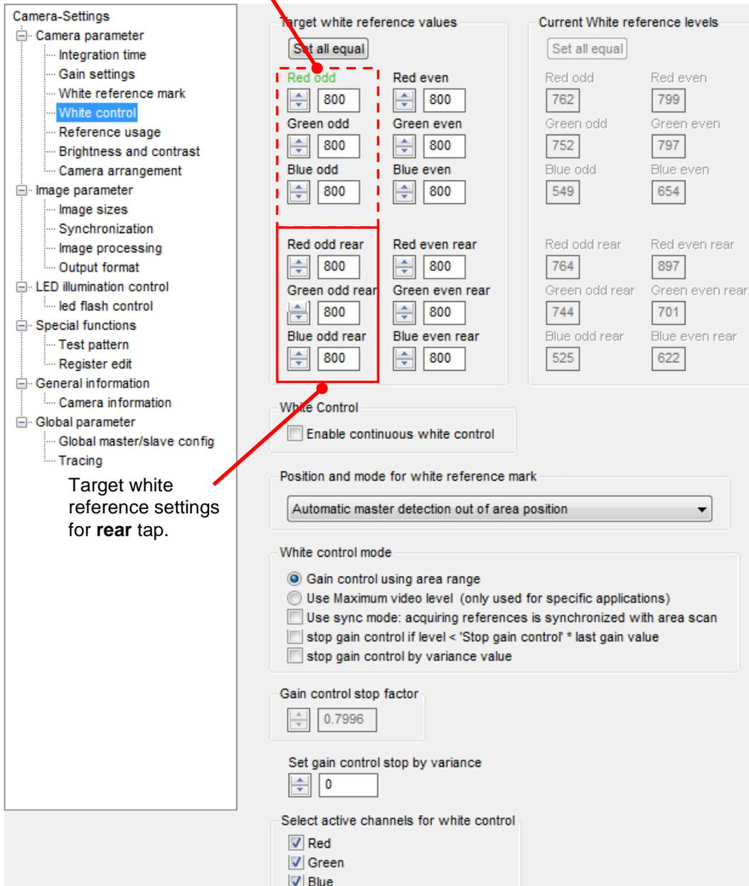
The screenshot displays the 'Camera-Settings' menu on the left and the 'White control' settings on the right. The 'White control' section is divided into 'Target white reference values' and 'Current White reference levels'.
