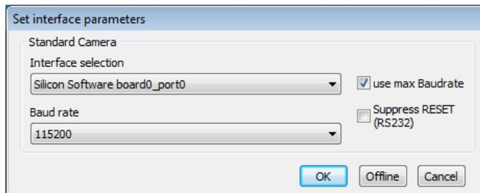
2. Select the PC interface for the communication either via Camera Link or external serial port.
