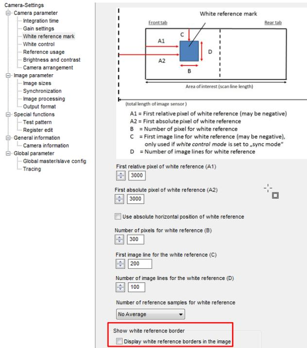
The screenshot shows the 'White reference mark' settings. A diagram at the top illustrates the 'Area of interest (scan line length)' with parameters A1, A2, B, C, and D. Below the diagram, the settings for A1, A2, B, C, and D are shown with input fields. At the bottom, the 'Show white reference border' section has the 'Display white reference borders in the image' checkbox checked, which is highlighted with a red box.
