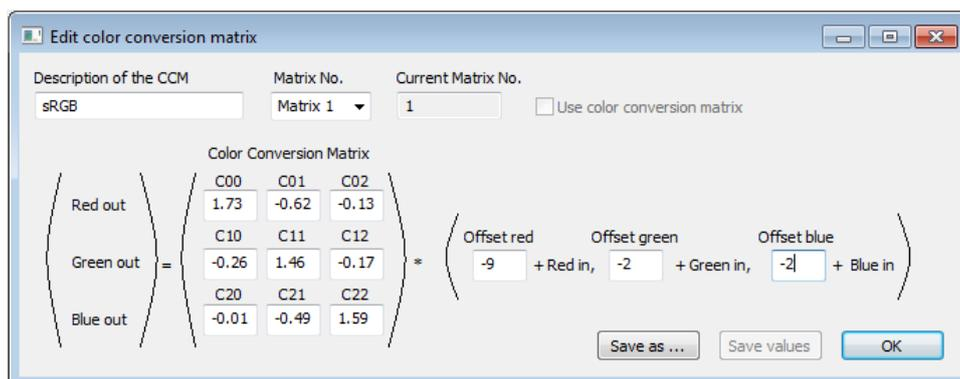
**NOTE** To use the sRGB conversion, additionally set **Gamma correction** to 0.1 on the **Brightness and contrast** page of the Camera Settings.
