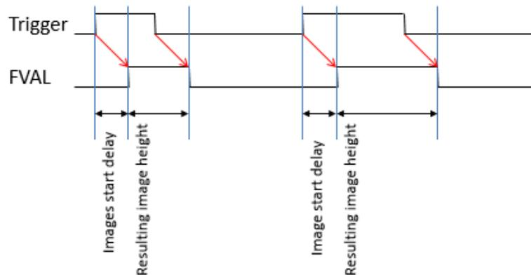
**Sample:** This function is useful for automatic detection of different object sizes; the camera sends a correctly sized image.
