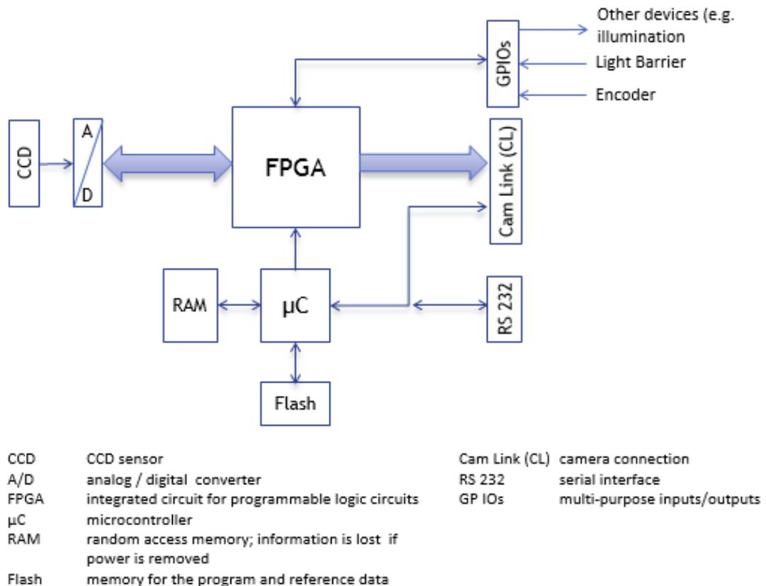
**Figure 4: Basic design of the allPIXA camera (block diagram)**
