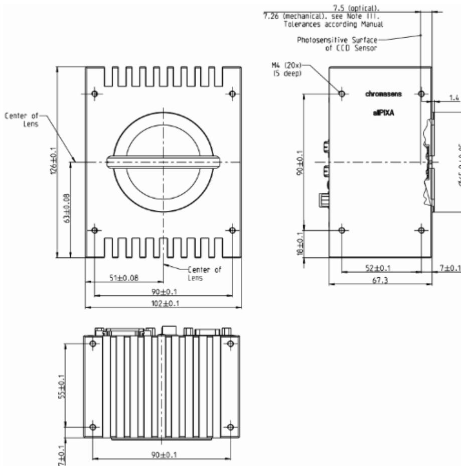
**Figure 3: Mechanical dimensions of the allPIXA camera with 7,300 pixels**
