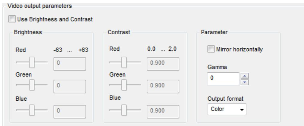
If the brightness and contrast parameters should be applied to the image, select the **Use Brightness and Contrast** check box. For more information about these parameters, see section 11.6.
