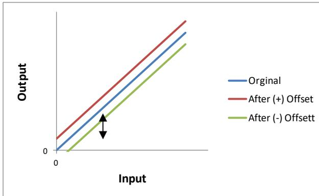
Take notice that using “Brightness” causes a digital offset in the image data:
