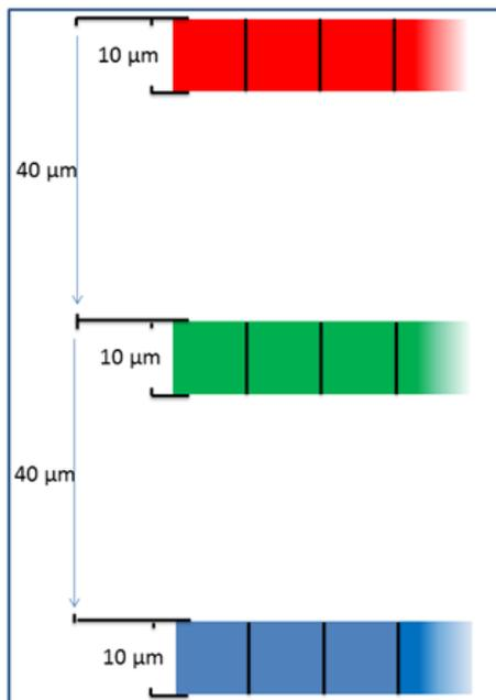
The allPIXA color line scan camera is equipped with a trilinear CCD line scan sensor with 3 spatially separated lines which are sensitive to the colors red, green and blue (RGB).
