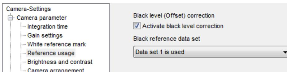
At least a few pixels should have a value greater than 0 (for example 1 or 2) in the black image with activated black-level correction and covered lens. Otherwise, (if **all** pixels are 0) the image is over-compensated and you should repeat the steps for reference generation.
