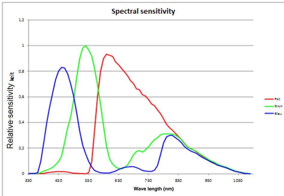
Figure 7: Spectral sensitivity of the line scan sensor
