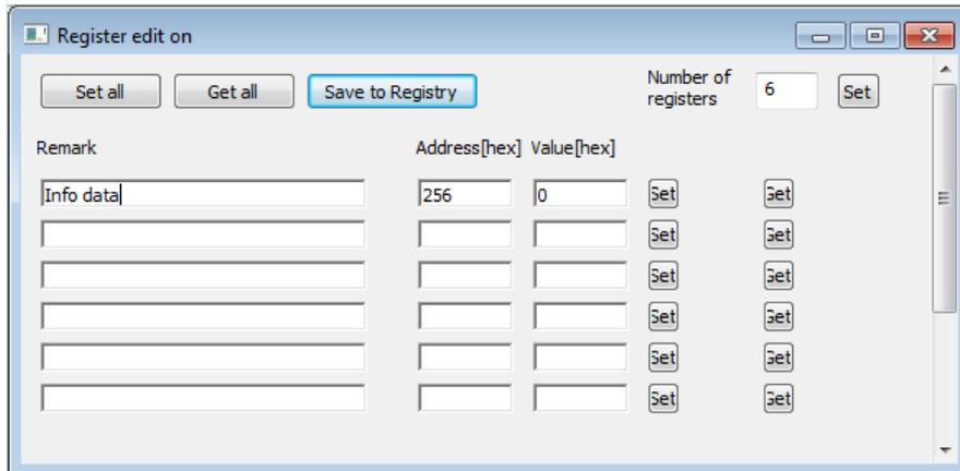
You can edit different registers directly. If you click **OK**, register names (**Remark**) and the address are saved on hard disk and are available for the next time.
