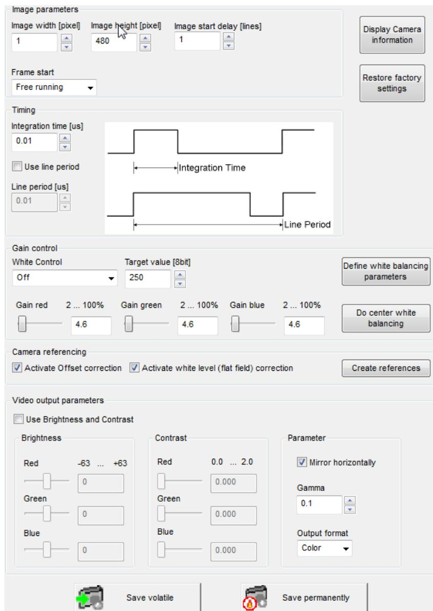
The screenshot shows the 'Simple setup view' interface for the allPIXA camera. It is organized into several functional sections:
