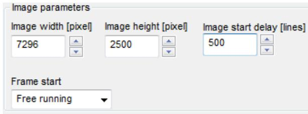
1. In the **Image width** box, enter the scan line length (see section 0).
