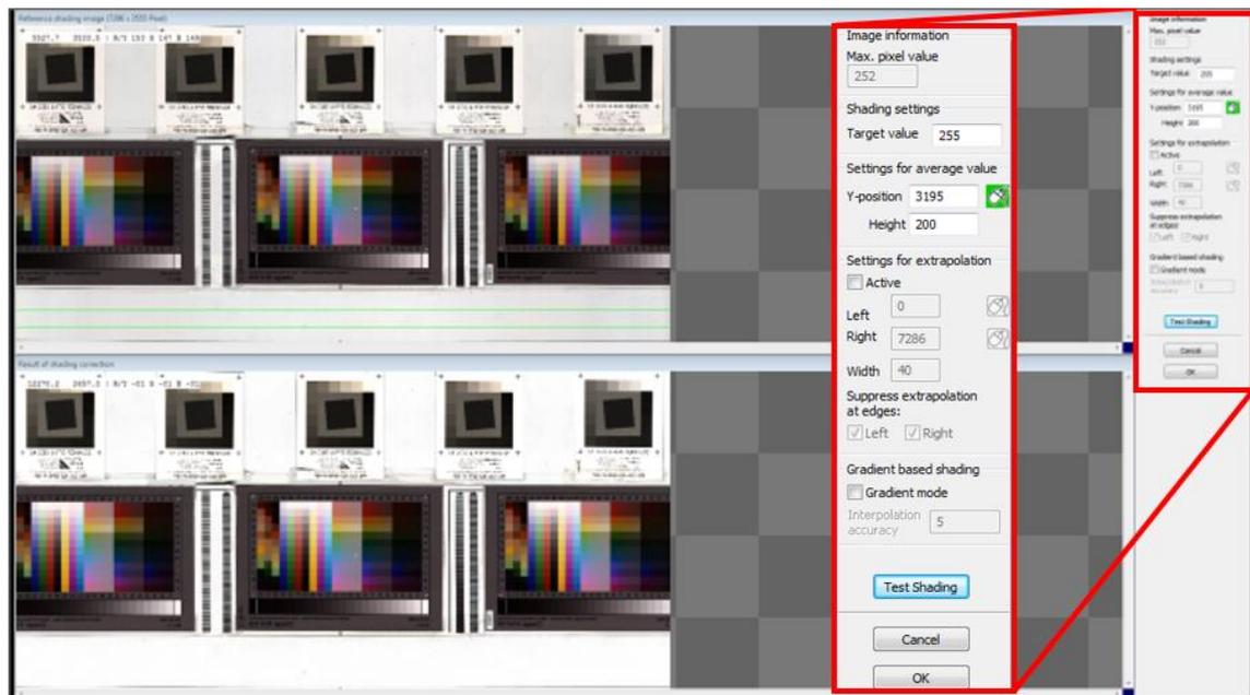
Use at least 100 lines for calculating the reference values to eliminate noise. The values used for the reference are calculated by averaging each column in the selected area.
