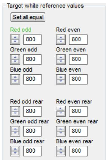
If the white target is placed at the borders of the image, they might be lower than in the center.
