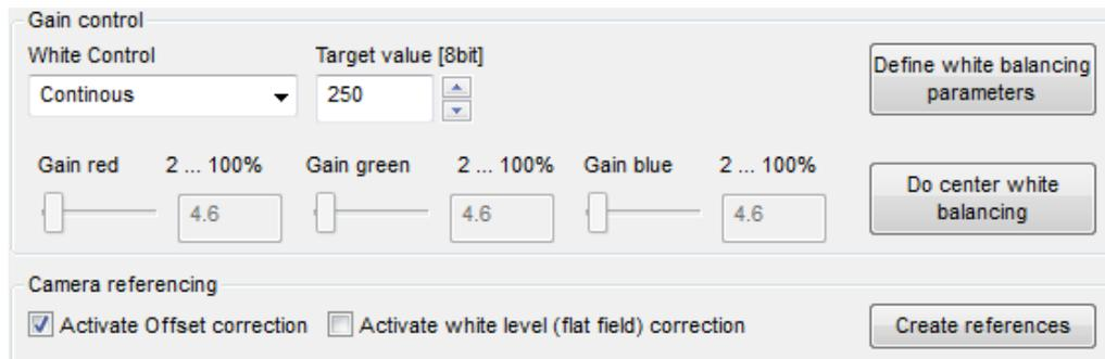
At the **White control** list specify, whether white control/balancing should operate continuously, only once per frame, or whether it should be switched off. If you select **Continuous**, the camera gain values are adjusted continuously during the scanning process.
