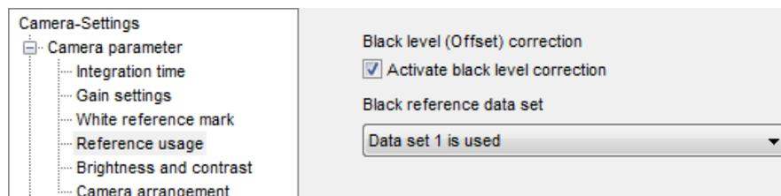
At least a few pixels should have a value greater than 0 (for example 1 or 2) in the black image with activated black-level correction and covered lens. Otherwise, (if **all** pixels are 0) the image is over-compensated and you should repeat the steps for reference generation.
