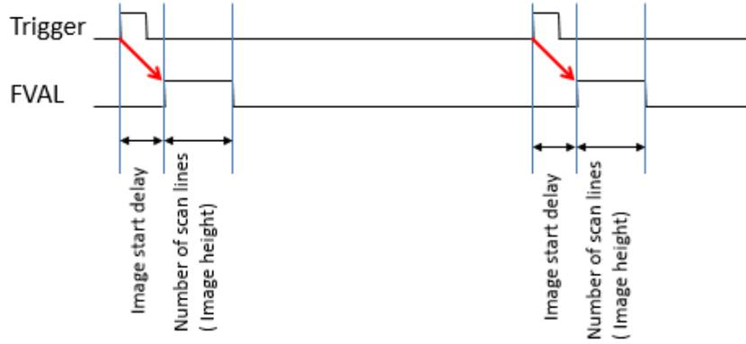
**Sample:** Image acquisition is started automatically. It is also possible to get a delay for a position of the light barrier before getting the scanning position.
