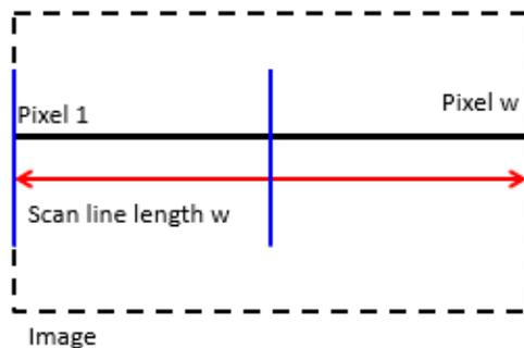
Scan line length is set to the sensor length of the camera, for example 4096.
