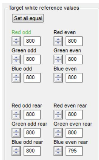
If the white target is placed at the borders of the image, they might be lower than in the center.
