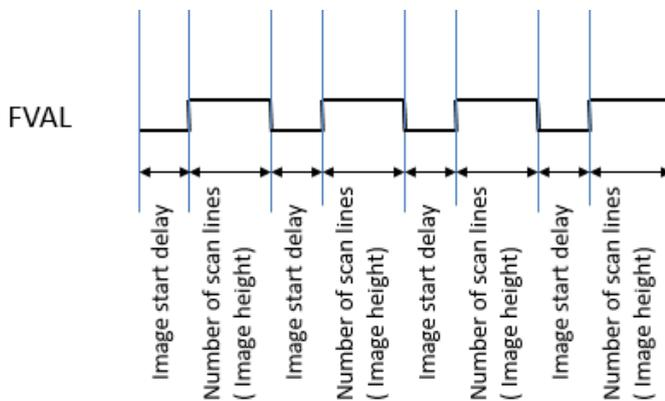
Sample for using Image start delay:
