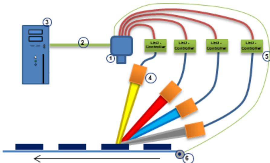
**Figure 25: Connecting flash controllers and illumination modules**
