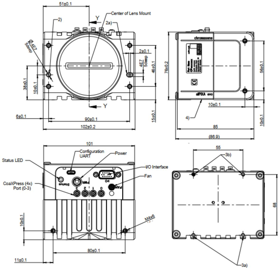
Figure 35: allPIXA evo 8k camera (CoaXPress interface, Y variant)
