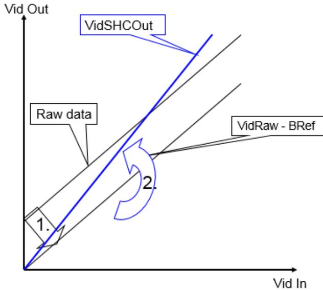
**Figure 11: Offset and shading correction**
