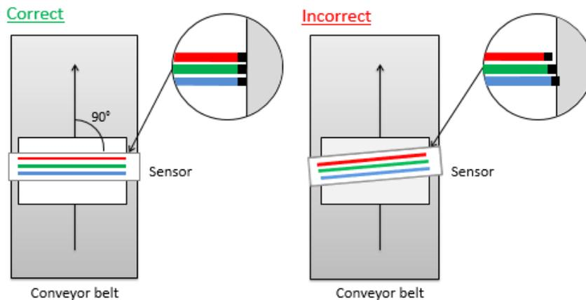
**Figure 19: Rectangularity of the sensor to the object**
