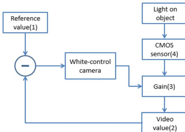
**Figure 12: Closed-loop control for white balancing**
