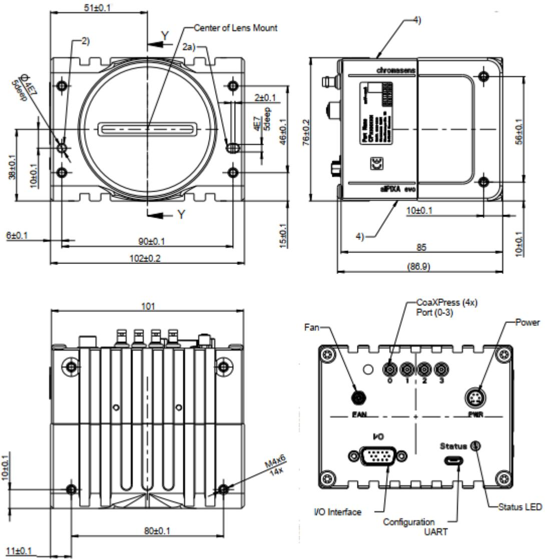
**Figure 36: allPIXA evo 8k camera (CoaXPress interface, Z variant)**
