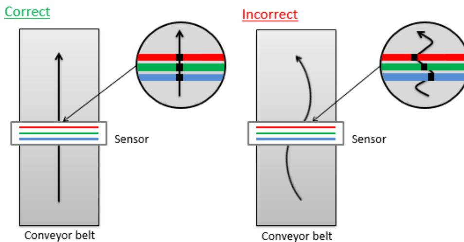
**Figure 18: Optimum conveyor belt tracking**
