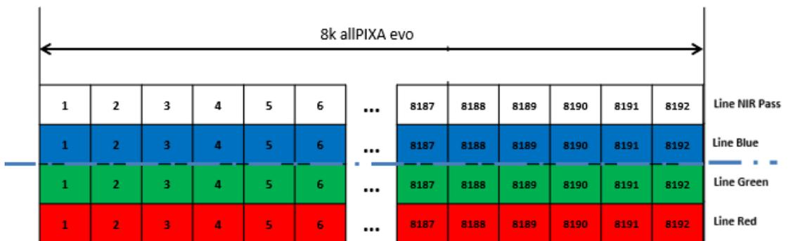
Figure 8 Pixel arrangement at the 8k allPIXA evo camera
