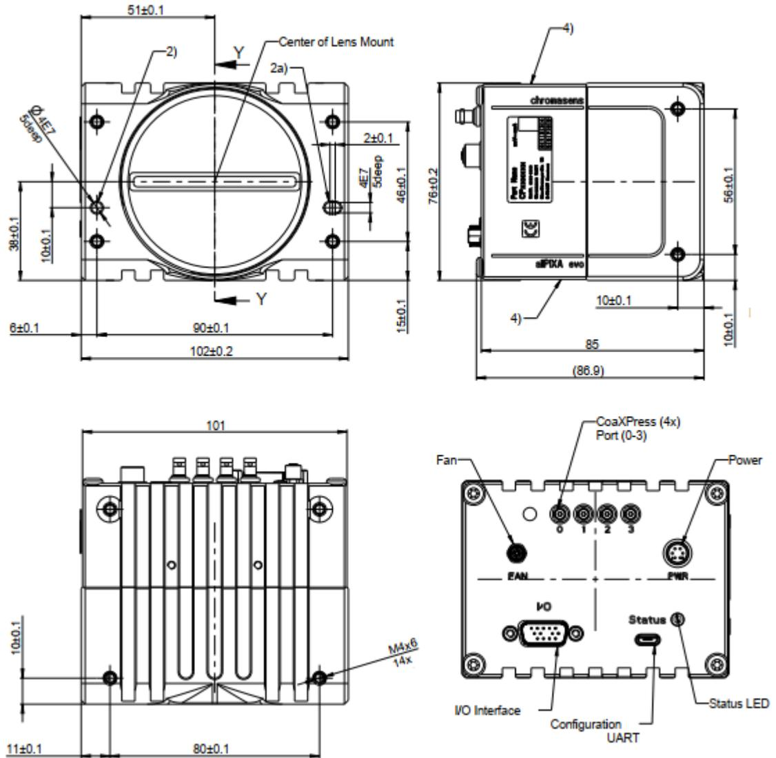
Figure 30: allPIXA evo 10k camera (CoaXPress interface, Z variant)
