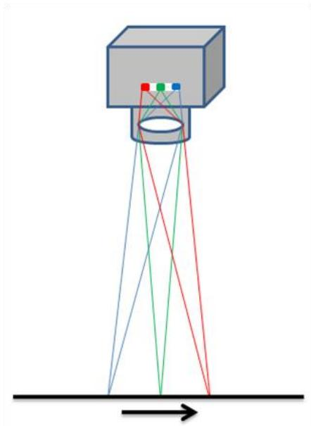
The 10K and 15K allPIXA evo camera color line scan cameras are equipped with a tri-linear CMOS line scan sensor with 3 spatially separated lines which are sensitive to brightness and the colors red, green and blue (RGB).
