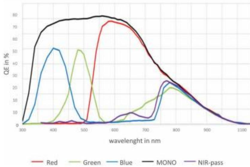
**Figure 9: Spectral sensitivity of the 8k line scan sensor (color and mono camera)**
