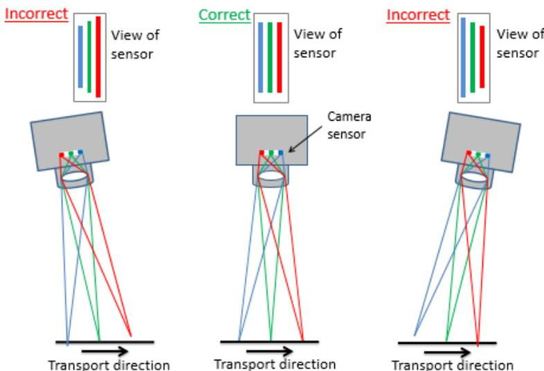
**Figure 20: Rotation around the longitudinal axis of the line sensor**
