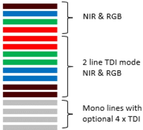
The 8K allPIXA evo camera color line scan sensor is equipped with a CMOS line scan sensor with 16 spatially separated lines which are sensitive to brightness and the colors.
