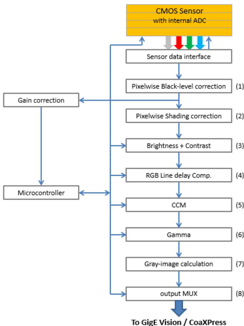
**Figure 10: Digital processing of the allPIXA evo camera (block diagram)**
