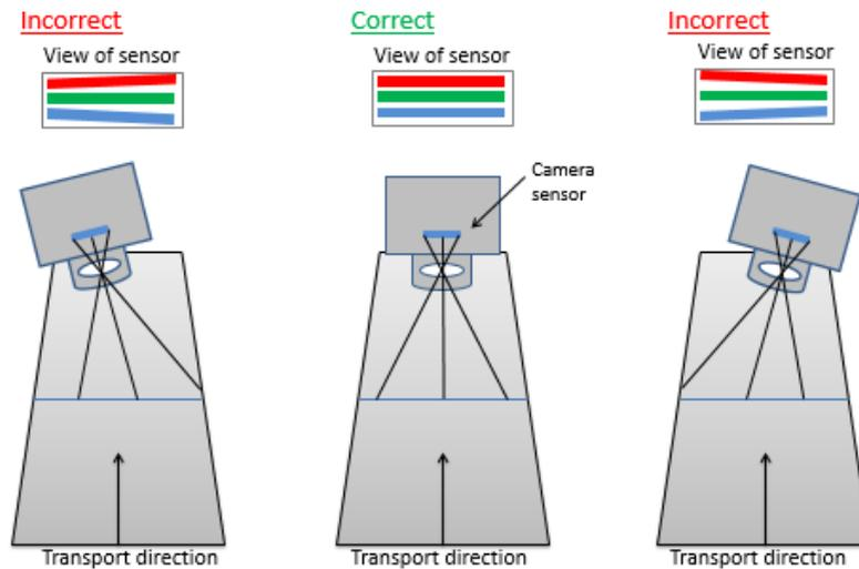
*Figure 21: Rotation around the transverse axis of the line scan sensor*
