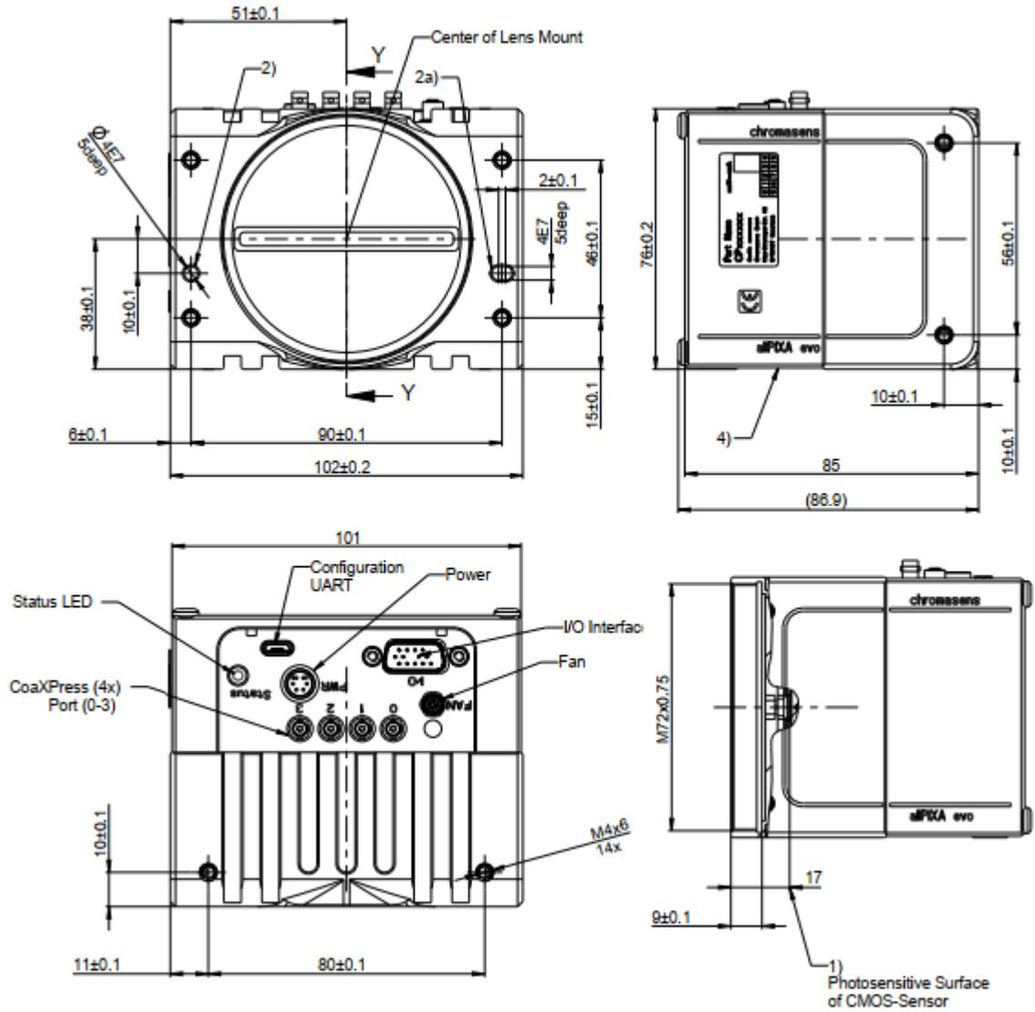
Figure 29: allPIXA evo 10k camera (CoaXPress interface, Y variant)
