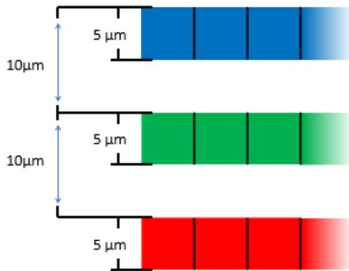
Sensor pixels are 5 μm wide and 5 μm long. The distance between the color sensor lines is 10 μm.
