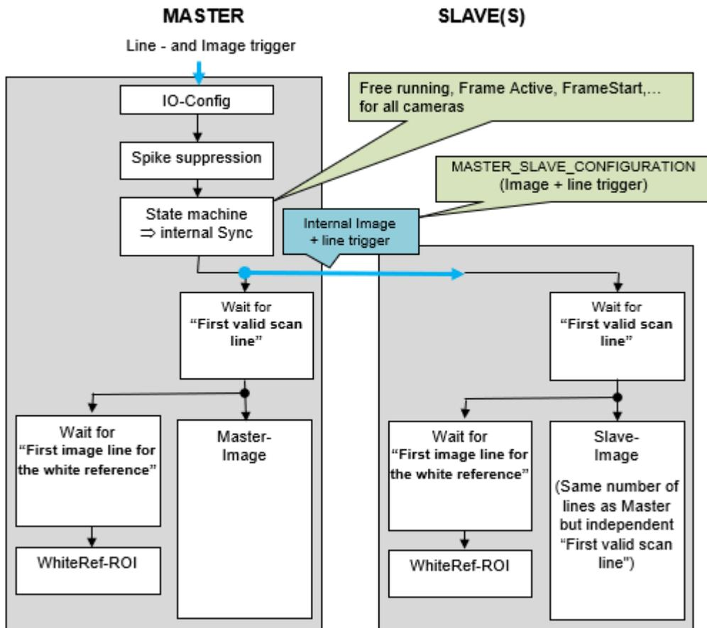
**Figure 27: Principle of master/slave mode**
